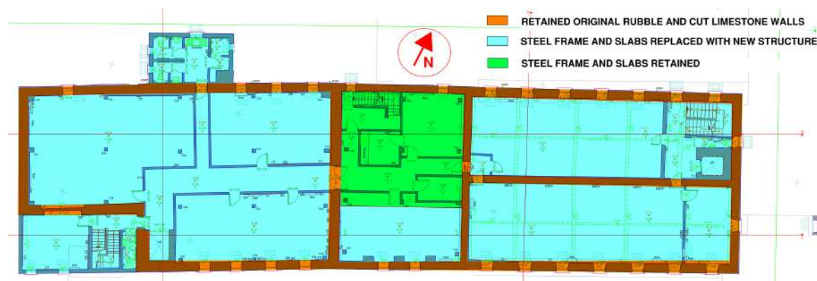
Figure 4.2 Level 1 structural interventions
