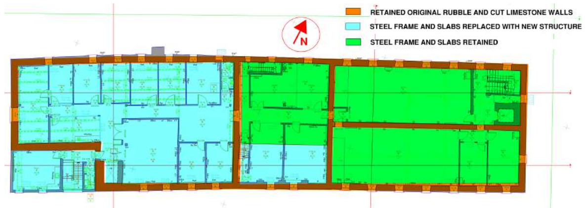
Figure 4.4 Level 3 structural interventions
