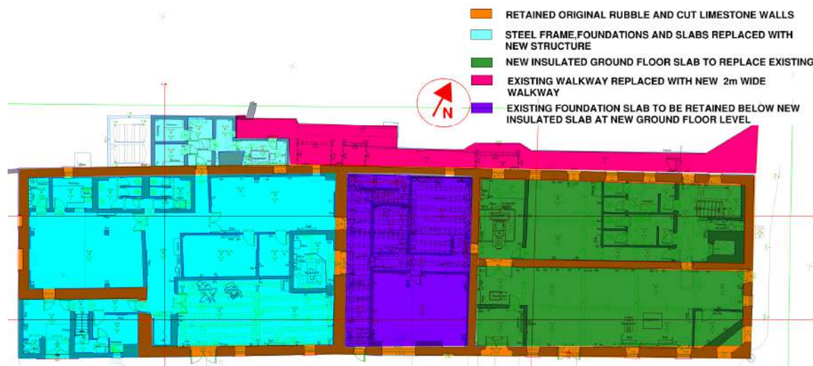
Figure 4.1 Ground floor structural interventions
